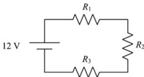
**Figure 12.5.** Series circuit
