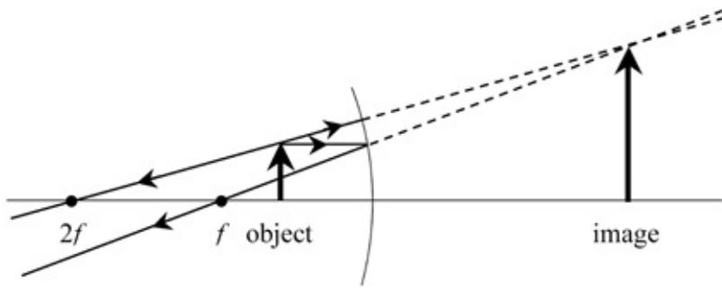
**Figure 16.12.** Virtual image in a concave mirror
