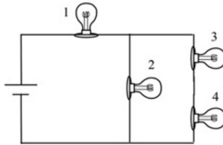
47. The lightbulbs connected in the circuit above all have identical resistances. Rank the light bulbs in order from brightest to dimmest.
