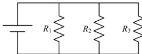
Figure 12.6. Parallel circuits
