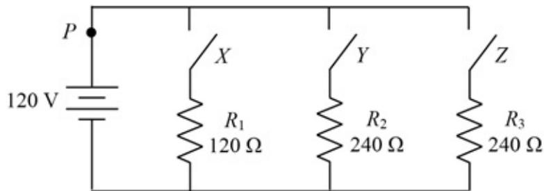
48. What current is following through point  $P$  when switches  $X$  and  $Y$  are closed?
