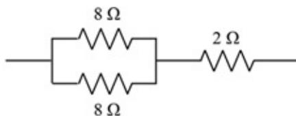
46. What is the equivalent resistance for the portion of the circuit shown in the above diagram?
