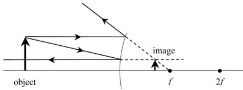
**Figure 16.13.** Diverging convex mirror
