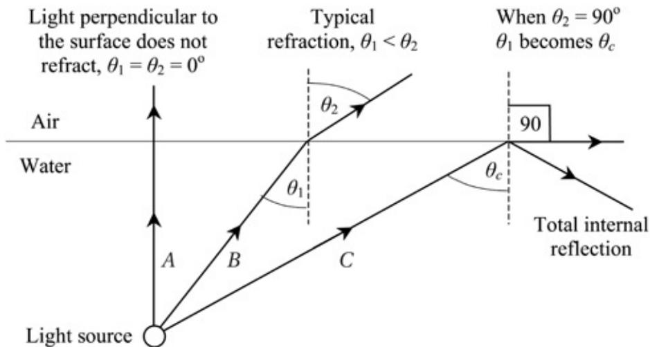
Figure 16.5. Total internal reflection
